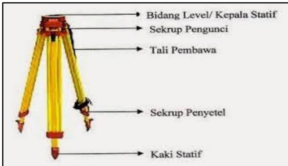
Gambar 3.8 Tripod Statif *Waterpass*
