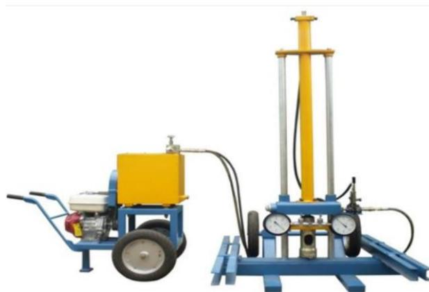
Gambar 3.7 Alat Sondir
