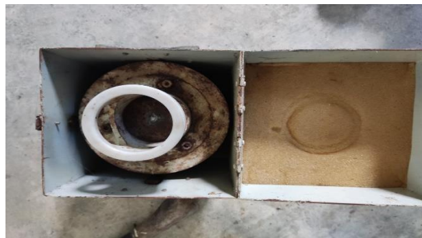
Gambar 3.7 Calibration Anvil Hammer Test
